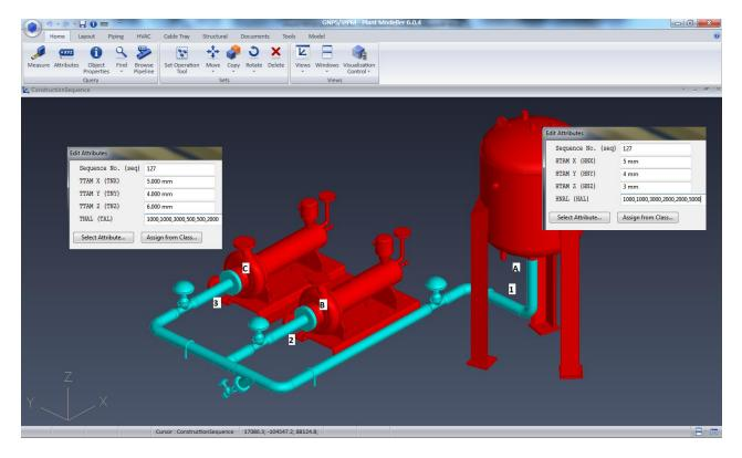
User can also add / modify the Thermal Anchor Movement values through Edit Layout option. i.e., Click Edit Layout then select "Anchor" and select "Edit data" through Layout > Edit. From the dialog box shown, click on "Specified Displacement" and enter the TAM values.
