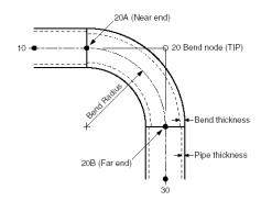
Node 20 is the Bend node, which is at the Tangent Intersection Point (TIP). As you can see from the figure, TIP is not physically located on the bend. Its only purpose is to define the bend. CAEPIPE automatically generates the end nodes of the curved portion of the bend (nodes 20A and 20B, called the near and far ends of the bend). The data items such as flanges, hangers, forces, etc. can be specified at the bend end nodes (20A and 20B in the figure).
