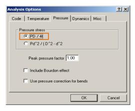
f. The analysis option in CAEPIPE corresponding to CAESAR II "Bourdon Pressure" is shown in figure right below.
