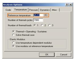
The analysis option in CAEPIPE corresponding to CAESAR II "use PD/4T" is shown in figure right below.
