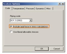
c. The analysis option in CAEPIPE corresponding to CAESAR II "Liberal Expansion Stress Allowable" is shown in figure right below.
