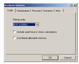
The analysis option in CAEPIPE corresponding to CAESAR II "Add F/A in Stresses" is shown in figure right below.
