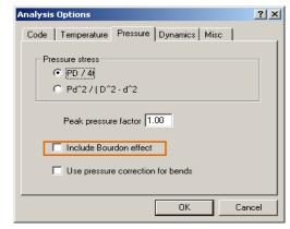
g. The analysis option in CAEPIPE corresponding to CAESAR II "Use pressure Stiffening" is shown in figure right below.
