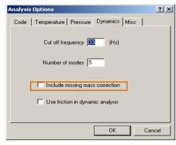
i. The analysis option in CAEPIPE corresponding to CAESAR II "Ignore Spring Hanger Stiffness" is shown in figure right below.
