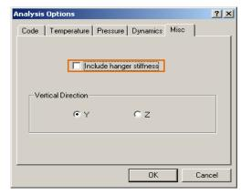
j. The analysis option in CAEPIPE corresponding to CAESAR II "Z-Axis Vertical" is shown in figure right below.
