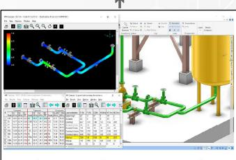
Detailed Analysis by Stress Engineer with 3D Plant Model in view
