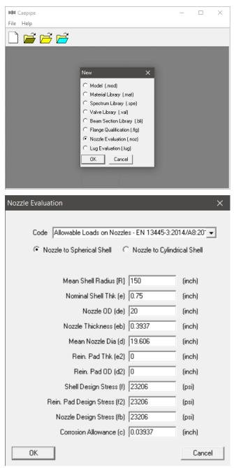
After entering the details, press the button "OK", save the model and perform the analysis through File > Analyze. This computes the allowable radial nozzle load as well as the allowable bending moment on nozzle welded to Spherical Shell. See snap shot below for details.
