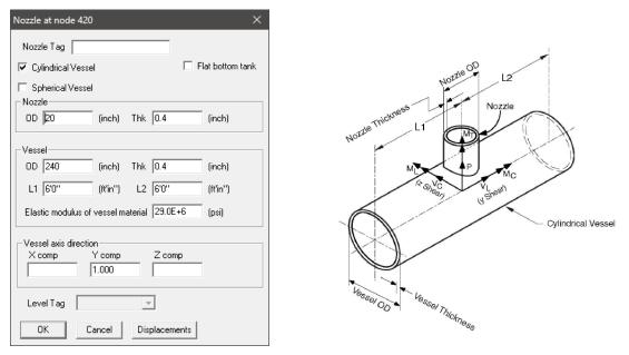
From the snap shot shown above, Lengths L1 and L2 on either side of the nozzle, which are the distances from the nozzle center line to the nearest location on vessel where the "ovalization deformation" of the vessel is stopped such as at a stiffener on the inner or outer surface of the vessel, or at the center of a saddle support to the vessel or at the junction to the torispherical enclosure (also called the head) or at a tube sheet inside the vessel etc.
