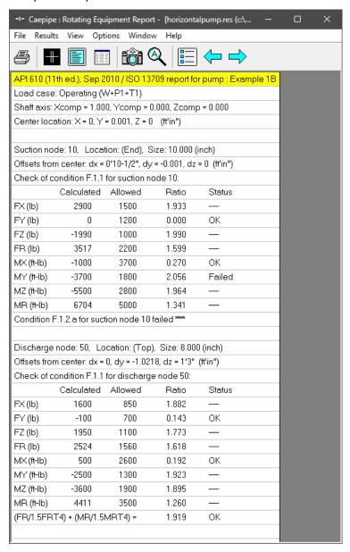
A similar procedure as described above can be followed for producing Compliance report for API 610 - Vertical Pump, ANSI/HI 9.6.2 Rotodynamic Pumps, NEMA SM-23 - Turbine and API 617 - Compressor.
