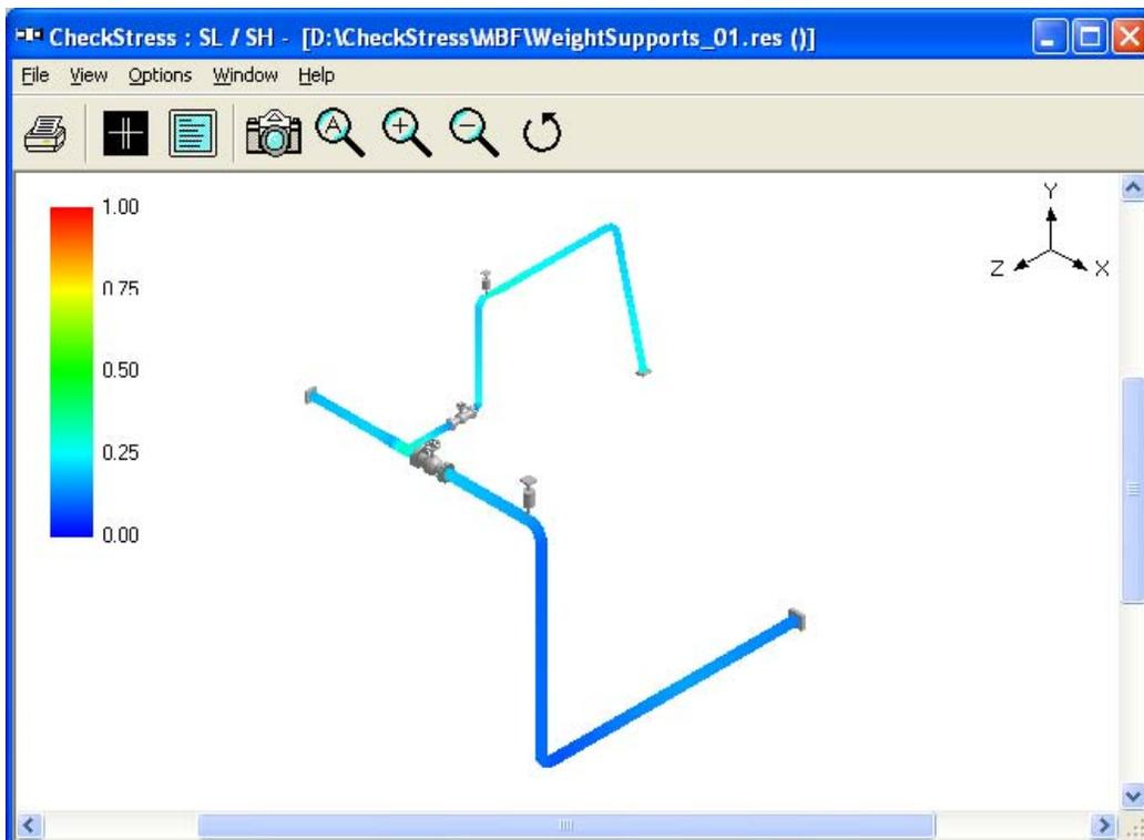
Figure 4G - Sustained Stress Contour Plot for Layout with Hangers
