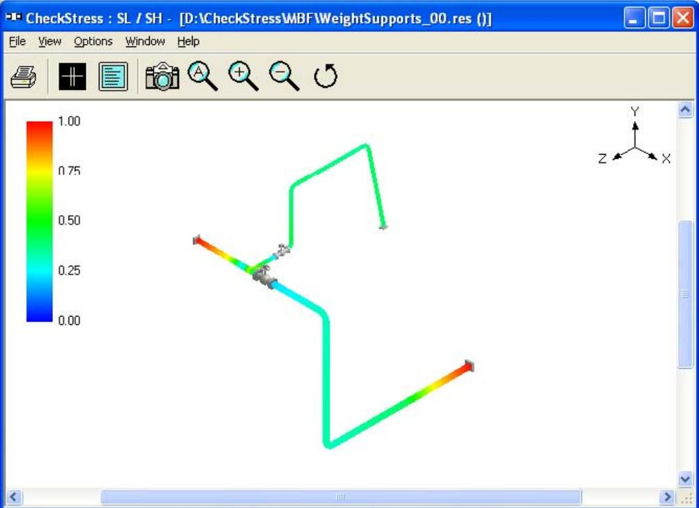
Figure 4D - Sustained Stress Contour Plot
