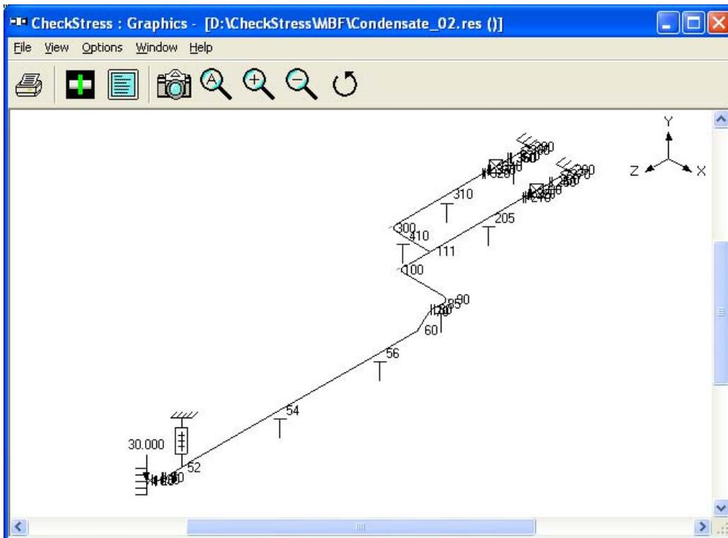
Figure 5H - Revised Layout with Resting Supports
