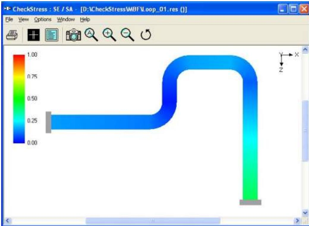
Figure 1E - (Code compliant thermal case)
