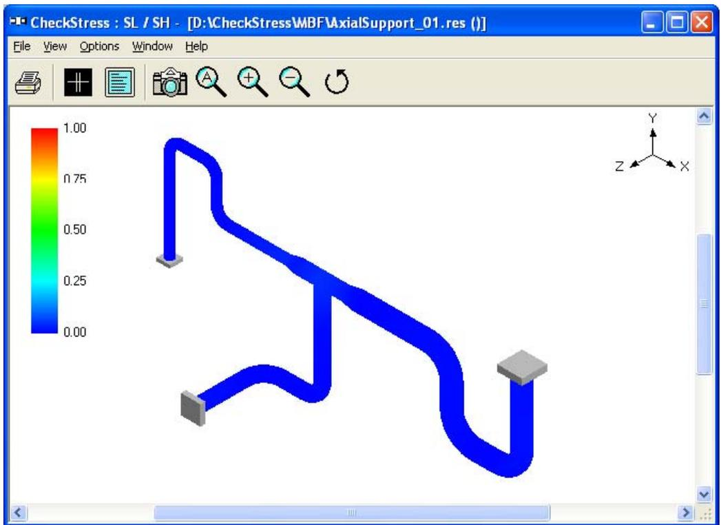
Figure 3G - Sustained Stress Contour Plot for Layout with Axial Restraints
