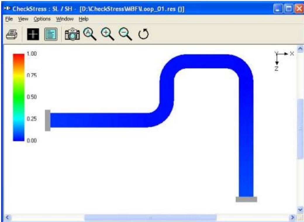
Figure 1F - (Code-compliant sustained case)
