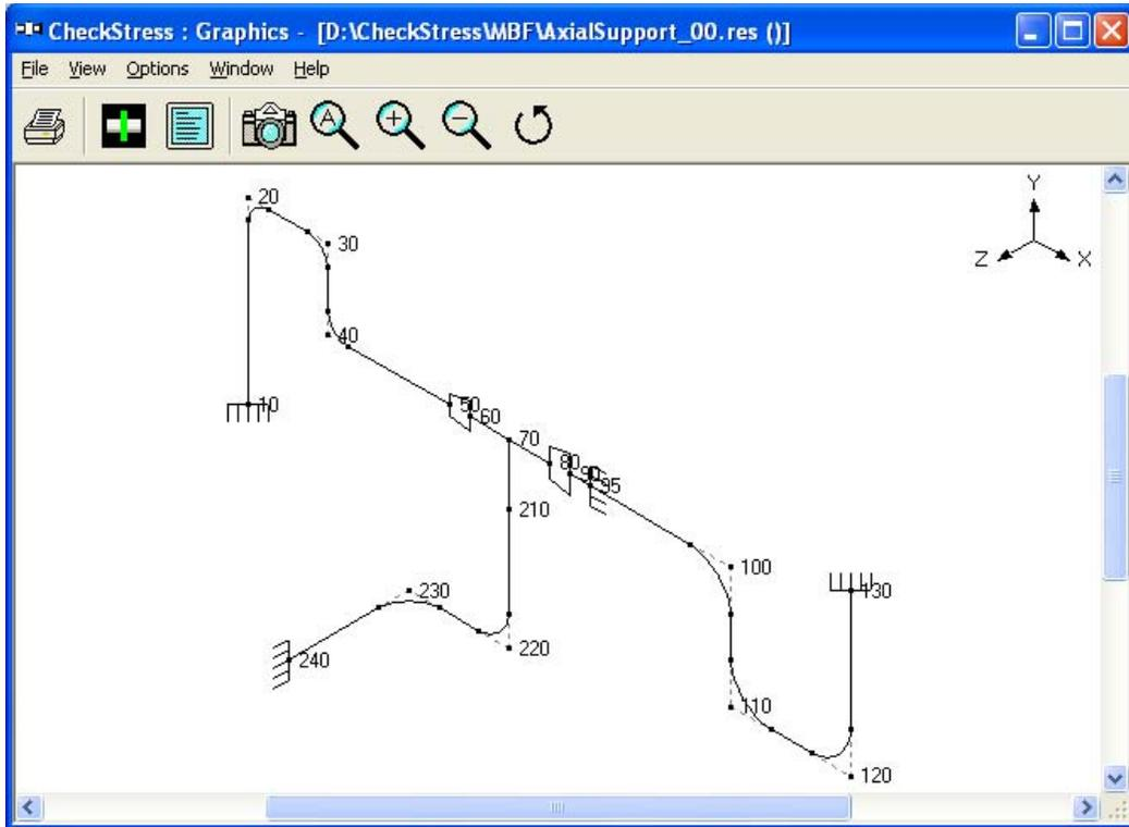
Figure 3A - Layout with Intermediate Anchor at Node 95
