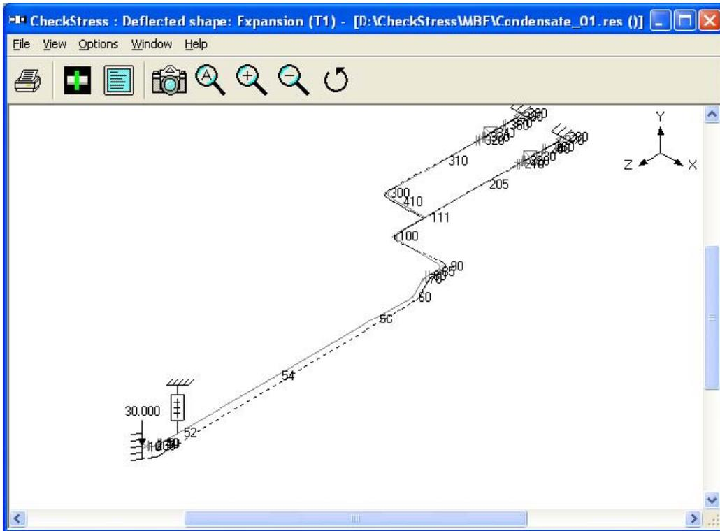
Figure 5E - Thermal Deformation Plot for Revised Layout
