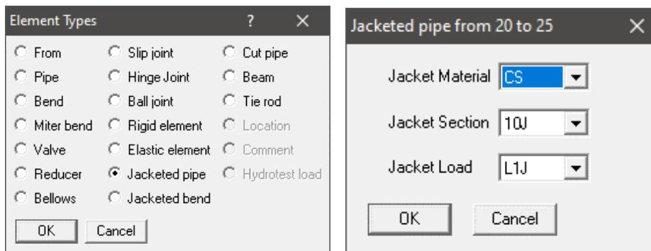
The jacket's material, section, and load names are input here (CS, 10J and L1J as shown). CAEPIPE retains the properties of a jacket pipe until changed so there is no need to retype the names of the jacket properties every time you input a jacketed pipe.
