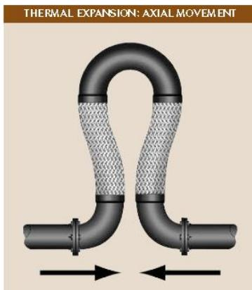
Illustrated above is a typical MetraLoop. No support is required for the 180° return bend for standard loops 2-1/2" diameter and smaller. However, due to the weight of the return bend and the extreme flexibility of the loop, larger sizes require support (as shown below) to prevent the loop from sagging in all orientations except when installed hanging down. Guides are recommended but not always required.
