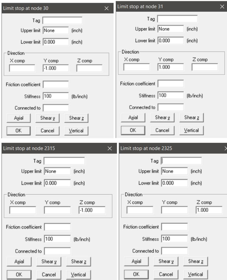
A limit stop in CAEPIPE prevents a node from moving beyond a certain distance (called a gap or a limit) in a certain direction. The node can move freely within the gap. After the gap closes, a limit stop acts as a rigid or flexible restraint (depending on your input for stiffness) resisting further movement of the node in the specified direction. If friction is specified, after the limit is reached, the friction force will oppose movement in the plane normal to the limit stop direction.
