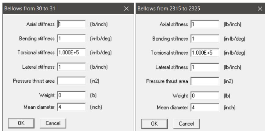
**Note:** Stiffness values should always be non-zero. In addition, for Flex hose, Pressure Thrust area should be entered as 0.0 or left blank.
