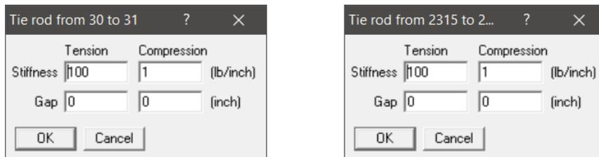
In this tutorial, since the Gaps in Tension and Compression are “0”, CAEPIPE will automatically use the Tension Stiffness as “100 lb/in” and Compression Stiffness as “1 lb/in” in analysis.
