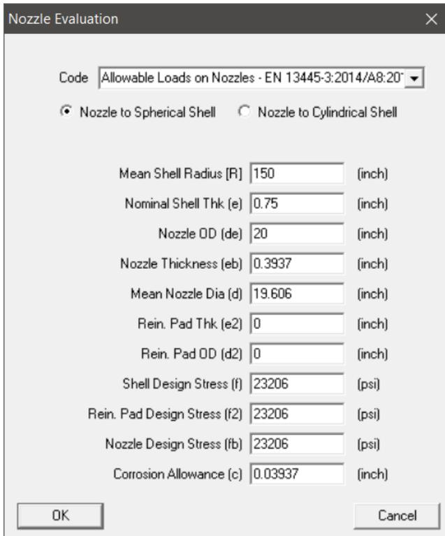
After entering the details, press the button “OK”, save the model and perform the analysis through File > Analyze. This computes the allowable radial nozzle load as well as the allowable bending moment on nozzle welded to Spherical Shell. See snap shot below for details.
