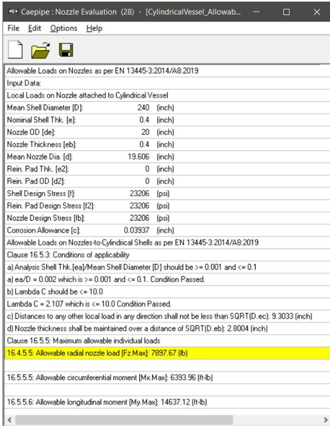
For both types of nozzles, the allowable loads in the two shear directions and in the torsional direction can be assumed to be very much larger than the corresponding allowable for the radial load and bending moment directions, as the shell is very stiff in those directions.
