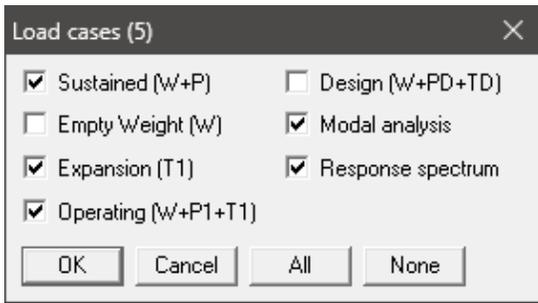
Upon analysis, CAEPIPE will show a “Load case” with name “Response spectrum” under “Support Loads”, “Displacements”, “Element forces” and “Support load summary” results.
